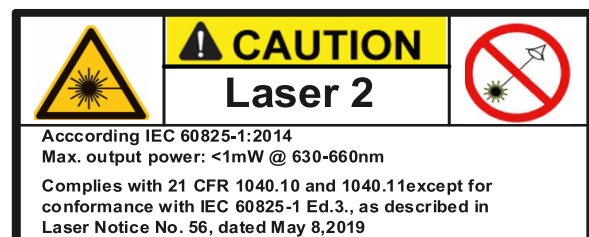
Figure 2: Product labeling "Class 2 laser"
